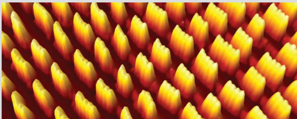
(*J. Phys. Chem. B* **110**, 21394–21398; 2006). Scanning tunnelling microscopy and low-energy electron diffraction revealed that the nanochains — which each contain just four or five fullerene molecules — only formed at the lower edges of the 'steps' that are found on the gold
