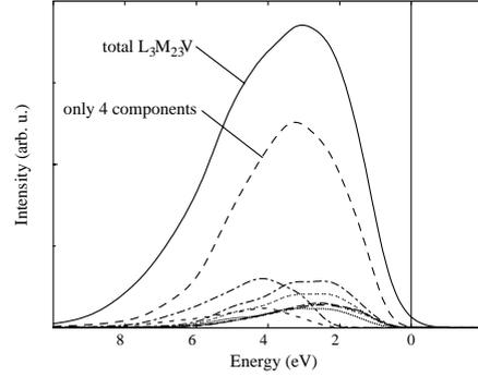
Fig. 1. Total (spin up + spin-down)  $L_3 M_{23} V$  AES of the surface layer of BCC Fe(100) (full line). Dashed curve is the sum of the four largest total partial AES. All other curves are the largest spin-resolved partial AES.
