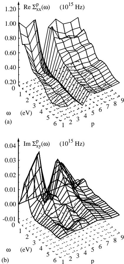
Fig. 2. Absorptive parts of the layer-resolved complex optical conductivity  $\Sigma_{\mu\nu}^p(\omega)$  for FCC(111)-Pt<sub>3</sub>|Co|Pt<sub>5</sub> as a function of the optical frequency  $\omega$  and the layer index  $p$ . Heavy line marks the Co-layer resolved optical conductivity  $\Sigma_{\mu\nu}^{p=1}(\omega)$ .
