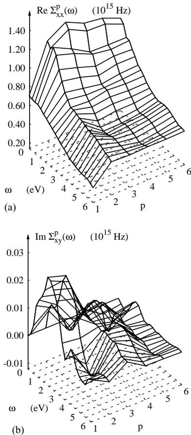
Fig. 1. Absorptive parts of the layer-resolved complex optical conductivity  $\Sigma_{\mu\nu}^p(\omega)$  for FCC(111)-Co|Pt<sub>5</sub> as a function of the optical frequency  $\omega$  and the layer index  $p$ . Heavy line marks the Co-layer resolved optical conductivity  $\Sigma_{\mu\nu}^{p=1}(\omega)$ .
