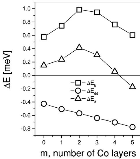
FIG. 3. Calculated band energy,  $\Delta E_b$  and magnetic dipole-dipole energy contributions,  $\Delta E_{dd}$  to the total magnetic anisotropy energy,  $\Delta E_a$  in  $\text{Cu}(100)/\text{Ni}_{13}(-5.5\%)/\text{Ni}_{17}(0\%)/\text{Co}_m$ .
