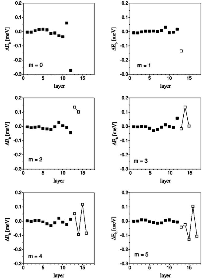
FIG. 2. Layer resolved band energy difference  $\Delta E_b^n$  for free surfaces of 0 to 5 Co layers on Ni(100)/Ni<sub>12</sub>(0%). Full and open squares denote Ni and Co layers, respectively.
