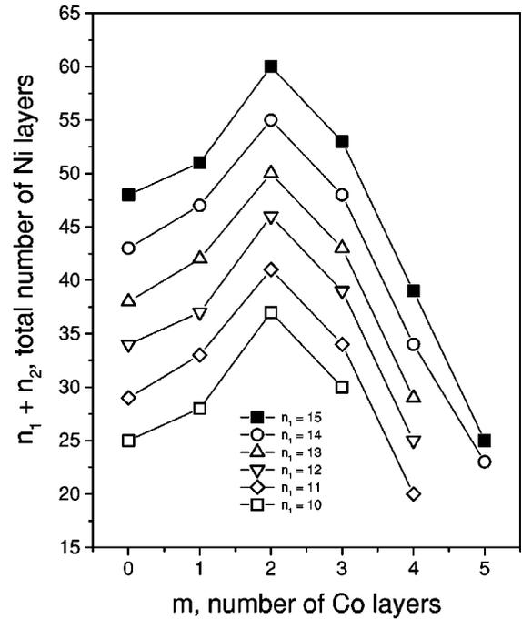
FIG. 4. Total number of Ni layers ( $n_1 + n_2$ ) at which the magnetic anisotropy energy,  $\Delta E_a$  of  $\text{Cu}(100)/\text{Ni}_{n_1}(-5.5\%)/\text{Ni}_{n_2}(0\%)/\text{Co}_m$  changes sign, displayed as a function of the number of Co layers ( $m$ ).
