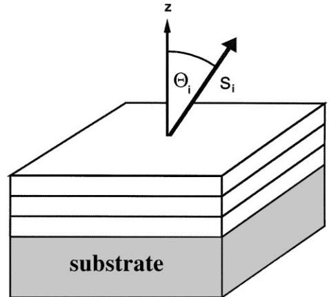
Fig. 1. Scheme of a thin magnetic film on a substrate displaying the convention used for the orientations of magnetization.
