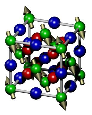
FIG. 1. Unit cell of the  $Ru_2MnZ$  full Heusler compound, with Ru atoms in red, Mn atoms in green, and Z atoms in blue. Golden arrows show the second kind of antiferromagnetic order (AF2) on the fcc sublattice of Mn atoms.
