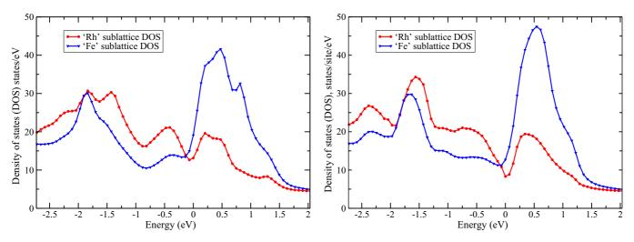
FIG. 2. (Color online) (a) Density of states of FeRh just above  $T_t$  in the F state,  $m_f = 0.59$ , and (b) just below  $T_t$  in the AF state,  $m_{af} = 0.71$ .
