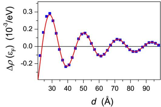
Fig. 4. Calculated difference of spectral functions,  $\Delta\rho(\epsilon_F)$ , (squares) with a corresponding asymptotic fit (solid line) as a function of the distance from the (001) surface of Au.
