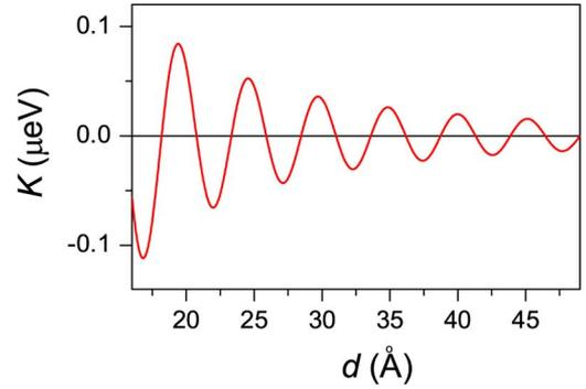
Fig. 3. MA constant within the HSO model as calculated from the asymptotic expression, (5).
