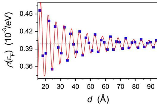
Fig. 2. Asymptotic fit, (3) (solid line), as function of the distance  $d$  from a Au(001) surface of the calculated off-diagonal spectral function,  $\rho(\epsilon_F)$  (squares), giving rise to the most significant contribution to  $\bar{K}(d)$  within the HSO model. The dashed line denotes the bulk value of  $\rho(\epsilon_F)$ .
