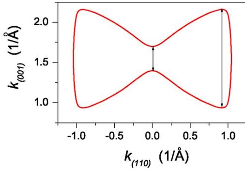
Fig. 1. Calculated plane cut of the FS of Au perpendicular to the  $(1 - 1 0)$  direction. The arrows denote the extremal vectors of the lengths,  $Q_{\min} = 0.298 \text{ \AA}^{-1}$  and  $Q_{\max} = 1.228 \text{ \AA}^{-1}$ .
