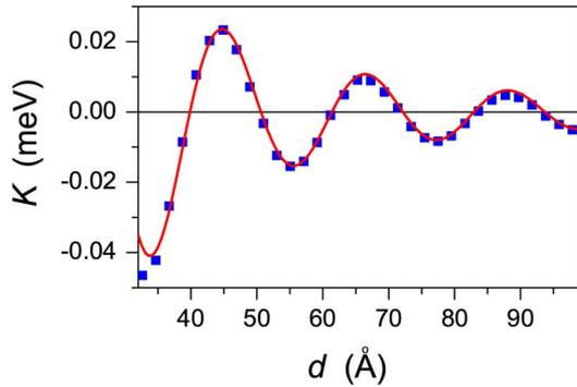
Fig. 5. MA constant within the LSO model calculated by using the asymptotic formula, (8), as a function of the distance  $d$  from the Au(001) surface (solid line). Squares stand for the MA constants calculated directly from (7).
