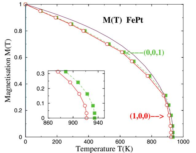
FIG. 1 (color online). The magnetization of FePt versus  $T$ . The filled squares refer to a magnetization along (0, 0, 1) and the open circles along (1, 0, 0).  $T_c$  is at 935 K with the easy axis, (0, 0, 1). The full line shows the mean field approximation to a classical Heisenberg model for comparison. In the inset, near  $T_c$ , the lower intercept shows what  $T_c$  would be with the system constrained to become magnetically ordered along (1, 0, 0).
