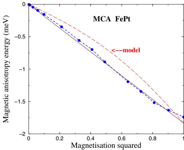
FIG. 2 (color online). The magnetic anisotropy of FePt as a function of the square of magnetization. The filled circles show the calculations from the *ab initio* theory, the full line  $K_0[M(T)/M(0)]^2$ , and the dashed line the single-ion model function  $K_0\langle g_2(\hat{e}) \rangle_T / \langle g_2(\hat{e}) \rangle_0$  with  $K_0 = -1.835$  meV.
