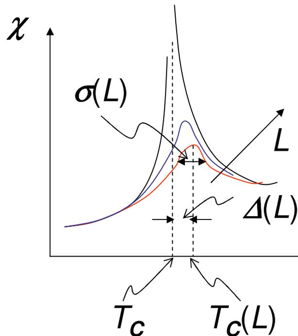
The deviation of the finite size behavior from that of the TDL is characterized by the shift  $\Delta(L)$  and the width  $\sigma(L)$
