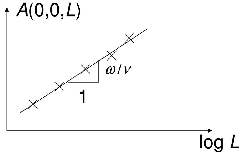
If precise enough data are available the scaling is not so nice: the lines on the log-log plots bend. This is because the simple power law scalings are valid only asymptotically and what we measure by linear fits are „effective exponents”. Since we can never reach „Asymptotia”, there will be corrections to scaling:
