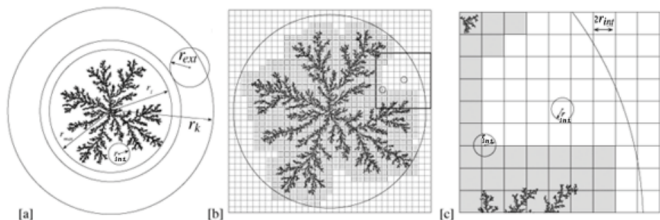
FIG. 1: (a) Schematic representation of the “optimized random trajectories”. (b) A DLA aggregate and a mesh of cells 2r_{int} \times 2r_{int} . Long steps are forbidden in the gray boxes and allowed in the white ones. Also, two long steps are illustrated. (c) A zoom of the region inside the large square in (b).
