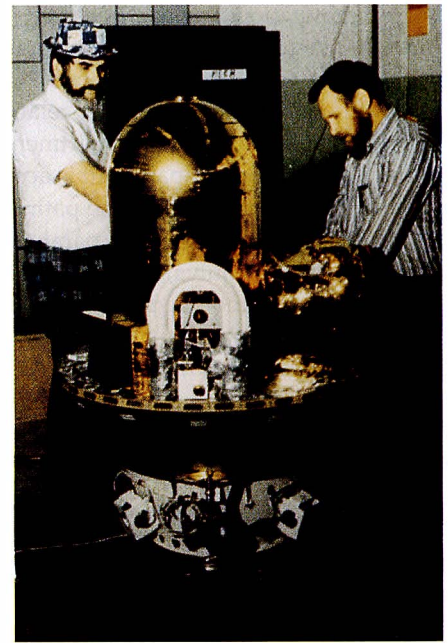
This extremely accurate hydrogen maser clock was launched in a satellite in 1976, and its time was compared to that of an identical clock on the earth. In accordance with the prediction of general relativity, the clock on the earth, where the gravitational potential was lower, lost approximately 4.3 \times 10^{-10} s each second compared with the clock orbiting the earth at an altitude of approximately 10,000 km.
